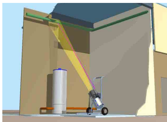
Figure 2 Using the ISOCS System to assay a pipe
