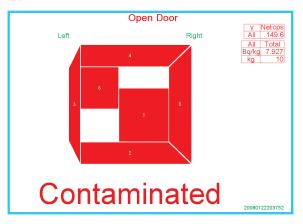
This display will show the quantity and location of the contamination based on which of the detectors is alarming, unless alarm is set on sum zone only. The operator opens the door, removes the object(s) and closes the door. The Cronos-1 will then perform a detector contamination check automatically to ensure there is no detectable amount of radioactivity remaining in the unit.
