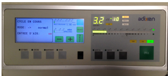
Leak rate < 1.10 -9 mbar.L.s -1 (He)
