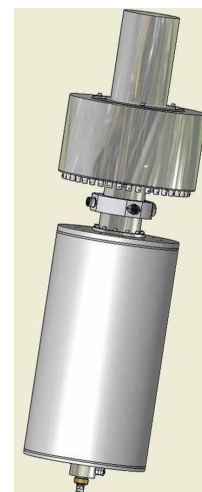
Coaxial 100% detector, segmented in 36 folds for tracking studies and pulse shape analysis.
