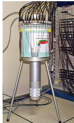
Mars (Mini Array of Segmented detectors) detector at Legnaro National Laboratories (Italy): 80% N type detector segmented in 25 folds.
