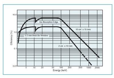
Absolute Efficiency Curve for LEGe Detector with 25 mm Spacing Between Source and End Cap
