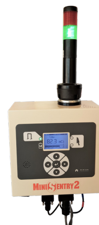
Readout unit with Light tower
