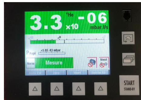
Leak rate < 1 . 10 -6 mbar.L.s -1 (He)
