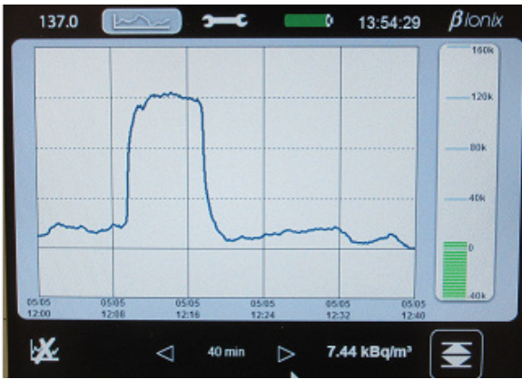
Example of the response at 100 kBq/m 3 B IONIX 3 – MES Volumetric activity measured
