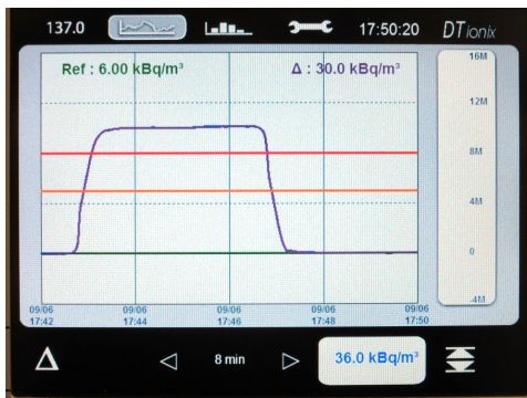
Injection of 10 MBq/m 3 (270 μCi/m 3 ) in a C IONIX 3 - BLC
