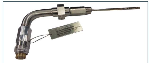
NSC with RTD (Resistance Temperature Detector)
