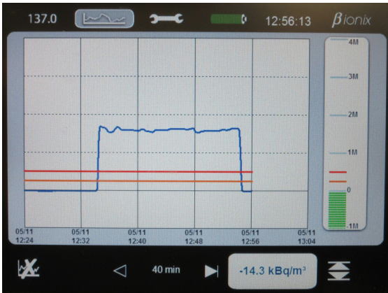
Response to a 1.6 MBq/m³ (43 µCi/m³) gas injection
