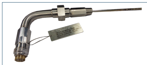
NSC with RTD (Resistance Temperature Detector)
