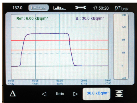
Injection of 10 MBq/m 3 (270 µCi/m 3 ) in a C IONIX 3 - BLC
