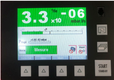
Leak rate < 1 .10 -6 mbar.L.s -1 (He)
