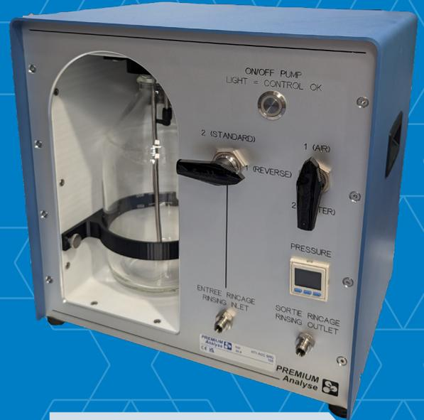
The HTI ACC SRD rinsing system helps prevent the creation of crystals in the bottles and/or the piping hence ensuring proper functioning and best availability of the HC IONIX carbon 14 bubbler. It can also be used, if needs be, to remove contamination in the tritium version of the bubbler.
