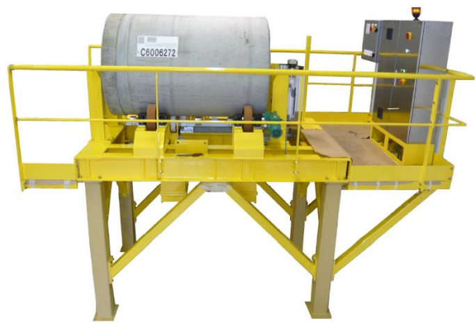
Automatic Hot Spot Localization on concrete drum
