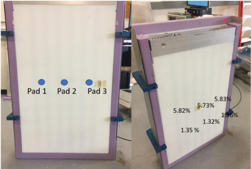
The blue marks indicate the measurement positions of the neutron source relative to each PAD (Pad 1, Pad 2, and Pad 3). The detection efficiencies were measured with the 252 Cf at distances of ≈0 cm and at ≈29.5 cm (six counter slab).
