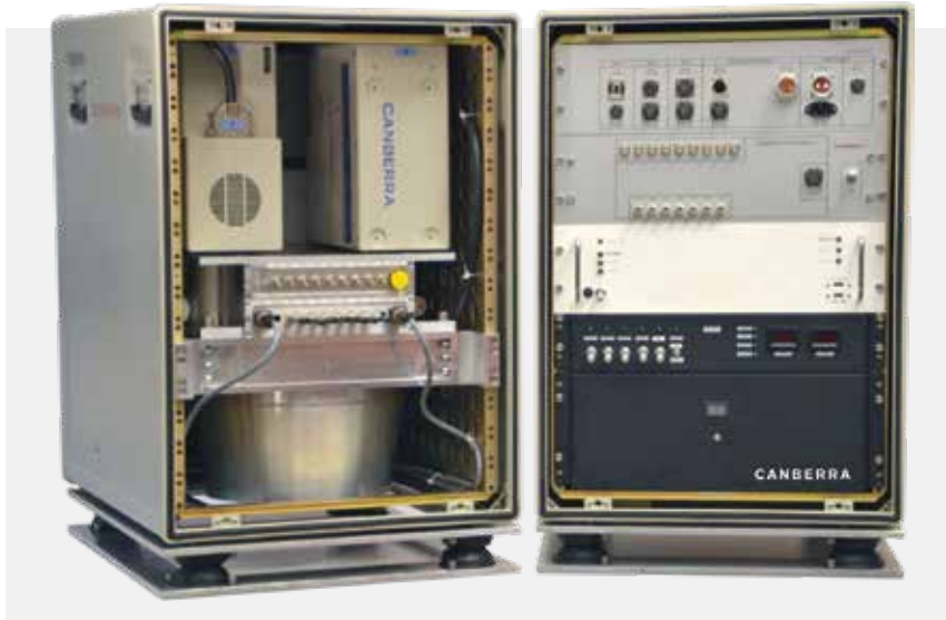
Hardware overview of the Mirion airborne system consisting of two cabinets (detector cabinet and acquisition system cabinet)
