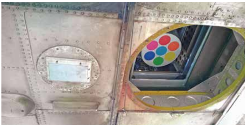
View of detector cap through a hole in aircraft cabin. Each colored circle shows the location of an individual coaxial detector within a common cryostat
