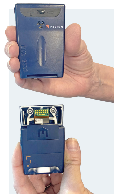
DMC 3000 Electronic Dosimeter with LTx module dedicated to Location and Telemetry
