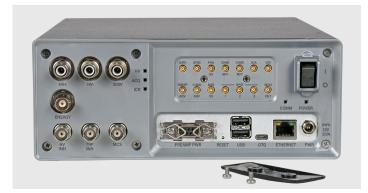
The system's versatility is augmented by its connectivity. For fast local or remote connections, the 10/100/1000 Base-TX Ethernet connection through the RJ-45 port or USB interface are optimal.
